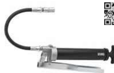
421/120 Mini lever operated grease pumps - Only for grease in bulk - Model with automatic grease feed - Feed pressure 413 bar - Tube diameter 36 mm - Supplied with flexible connection 300 mm and four-claw gripping tweezer - Threaded connection M10x1 - Steel body and lever
