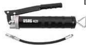
421 Lever operated grease pumps - Model with automatic grease feed to be filled from a bulk container or from a cartridge - Feed pressure 400 bar - Supplied with flexible connection 300 mm and four-claw gripping tweezer - Threaded connection M10x1 - Sheet steel body
